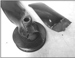
fan separated from the hub, damaging the hood with a loud "whack" and causing quite a shudder at 45 miles per hour. The car limped into Yreka where the fan was replaced with an old but sturdy, steel four-bladed fan, and the old, rattletrap is back on the road. The original fan broke along an old weld and the remaining, intact blade showed cracking at the hub. While Model A owners have long been warned about this potential failure, seeing is definitely believing.
